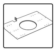
1. Nail or screw bracket to joists.
